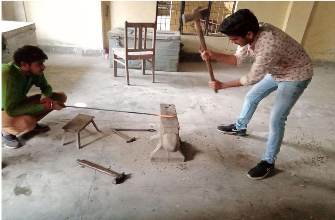
Fig. 2.23: A View of hammering process to cast the mild steel rod
