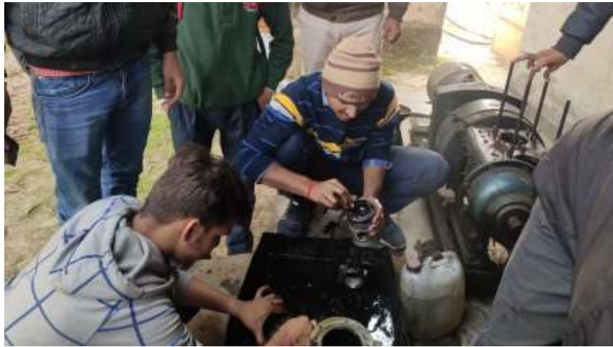
Fig. A view of dismantling of piston
