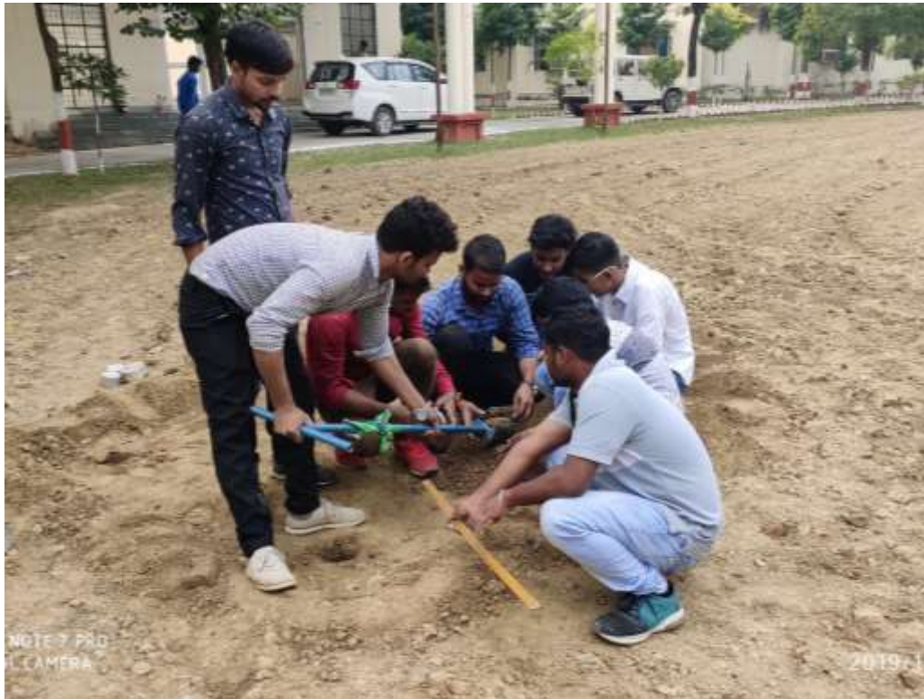
Fig. A view of collecting soil sample for determination of hydraulic conductivity
