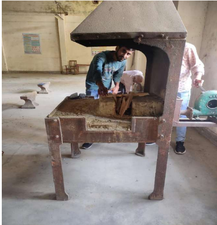
Fig. 2.10 (a): A View of Forging Furnace
