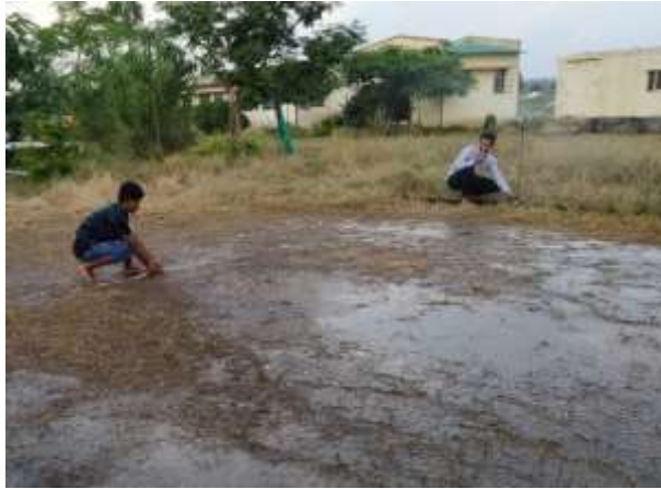
Fig. A view of coverage area measurement of rotating head type sprinkler head
