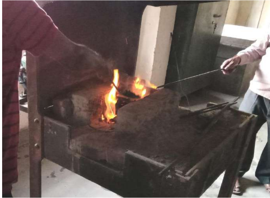
Fig. 2.21: A View of Putting Coal over the Tuyere
