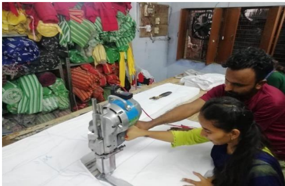
Students learning to use multi-layer fabric cutting machines at S.D. Hosiery centre, Ayodhya during In-plant training
