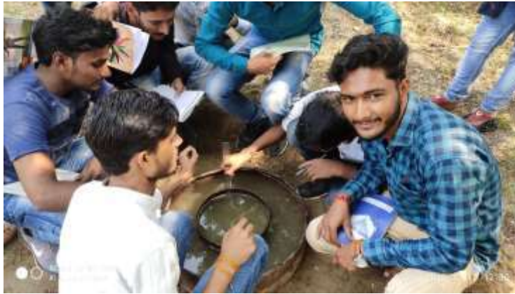
Fig. A view of taking a reading of infiltration rate
