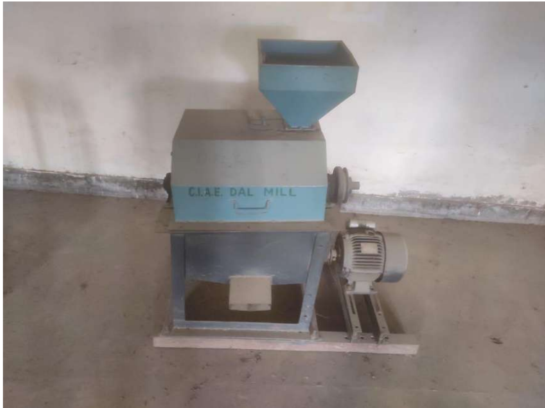
Fig. 2.5 CIAE dehusking and splitting machine
