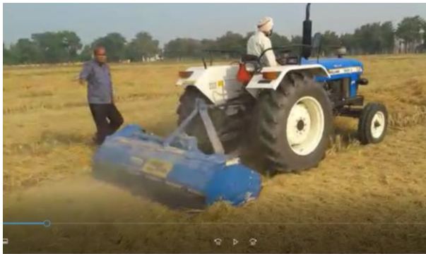
Crop Residue Management Using Power Shredder-cum-Mulcher at the University Farms
